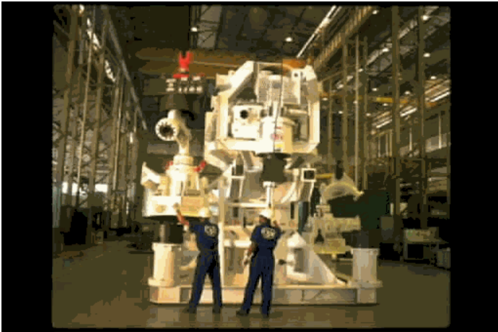
Figure A: Wet X-mas tree being readied for field installation.
